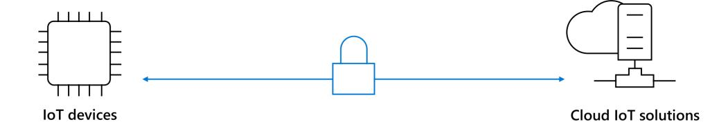
Tight coupling between software on device and IoT solution in the cloud
